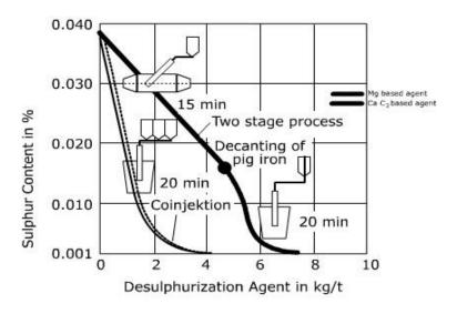
Figure1. Desulphurization of pig iron
