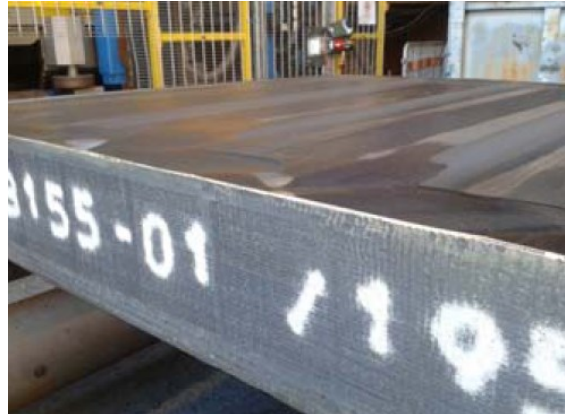
Figure 16. Longitudinal deburring grinding results
