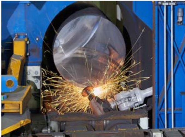
Figure 17. grinding robot in operation
