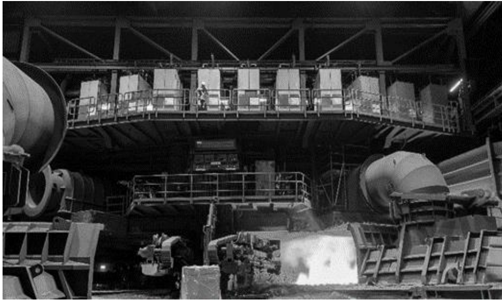
Figure 3: Image of tkse BF1 SIP boxes, located on a platform above the tuyere level.
