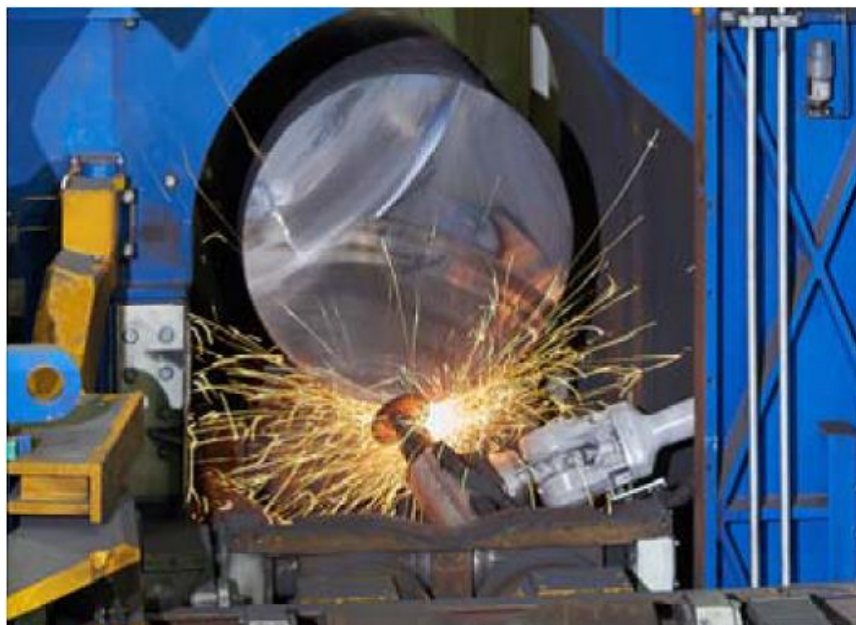
Chamfering grinding of head end of remelt ingot after cutting
