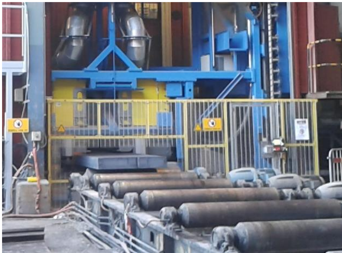
View on outlet area of deburring grinding facility
