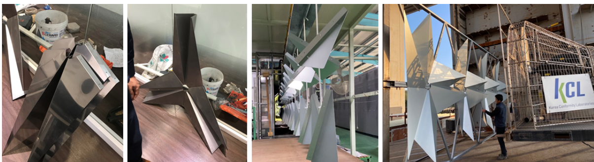
[Figure 10] Separated Panel Unit, PVDF Coating, Wind Pressure Test
