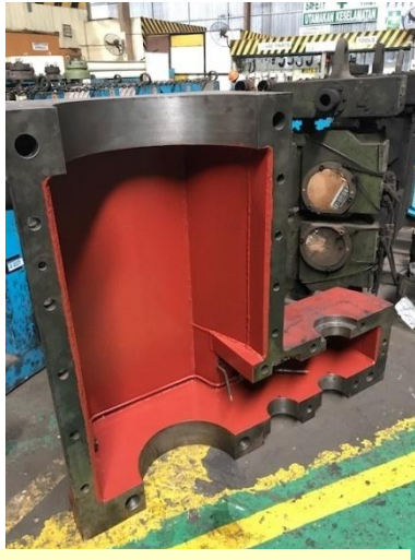
CLEANING OF GEARBOX CASING
