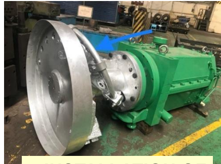
INSTALLATION OF ROTOR WITH PIPE
