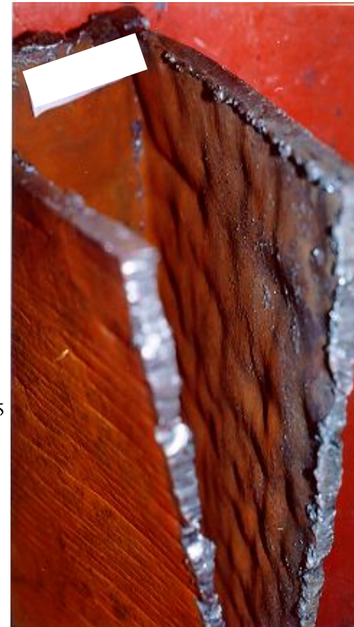
Hypo-peritectic carbon steel longitudinal crack formation breakout shell
