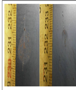
Fig. 1 Sliver defect on hot-rolled coil of peritectic steel.
