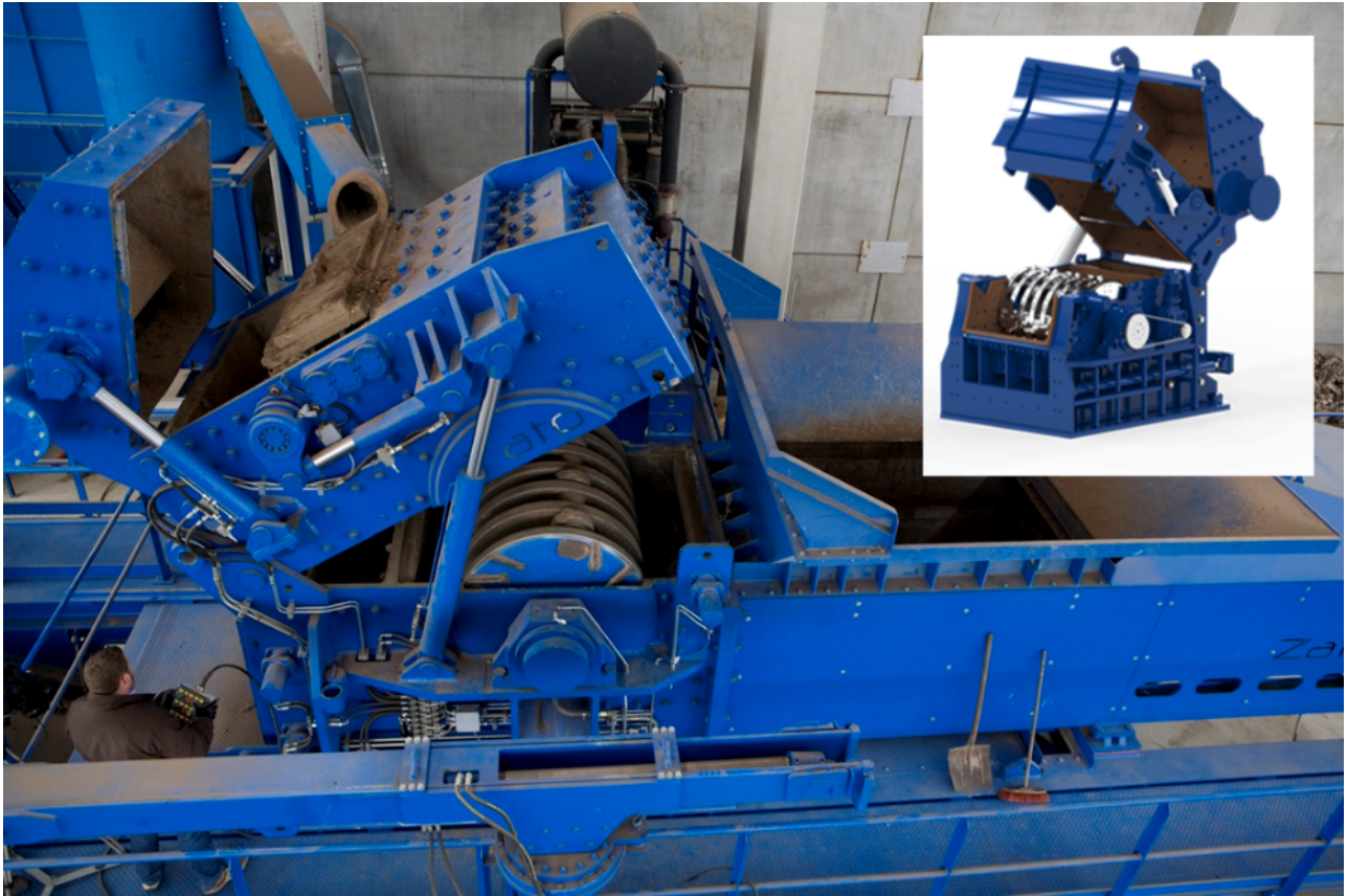
Figure 4 Hammer Mill Shredding Chamber with Rotor inside (Source Zato)
