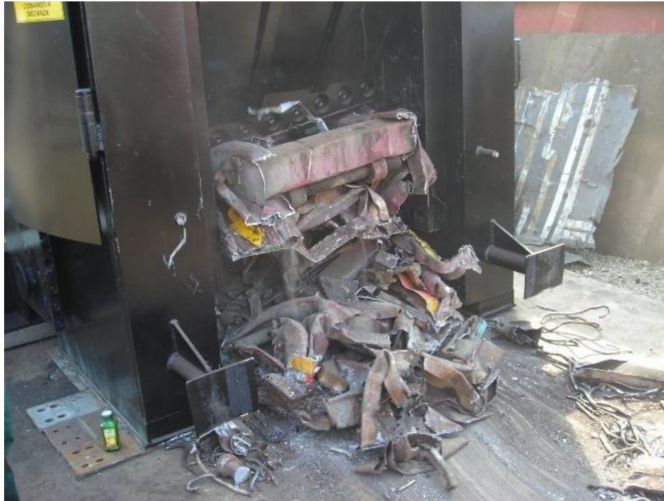
Figure 3. Head of the shear equipped with the blade
