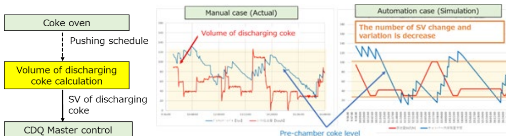
Figure 1-7 Optimum discharging coke volume by linkage with coke oven Source: Compiled by Nippon Steel Engineering
