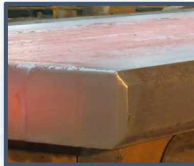
Chamfered slab \sim 818^{\circ}\text{C} (IR Sensor)
