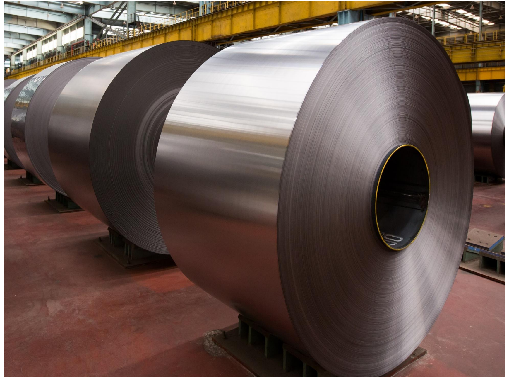
Source: worldsteel.org: Cold rolled coils in the storage yard (ID 31346), as per 16.10.2022
